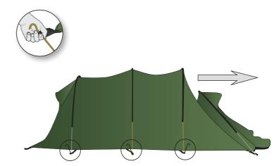
Mount the inner cabin in the O-rings and hooks. When you pack the tent, you can choose to leave the inner cabin attached.
